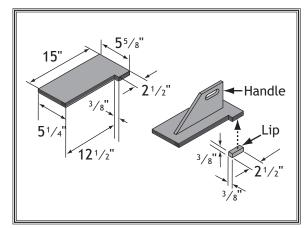
**Figure 77.** Push block dimensions and construction.
